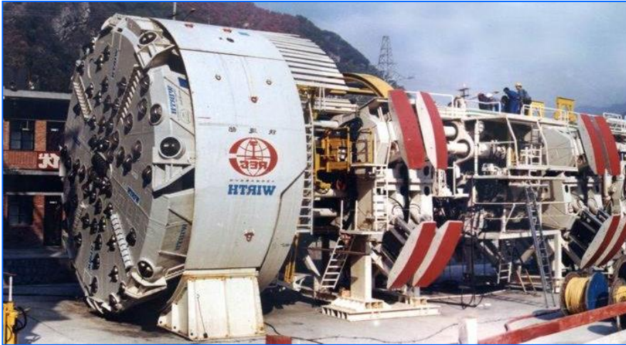
The TBM for the Xikang Qinling Tunnel
